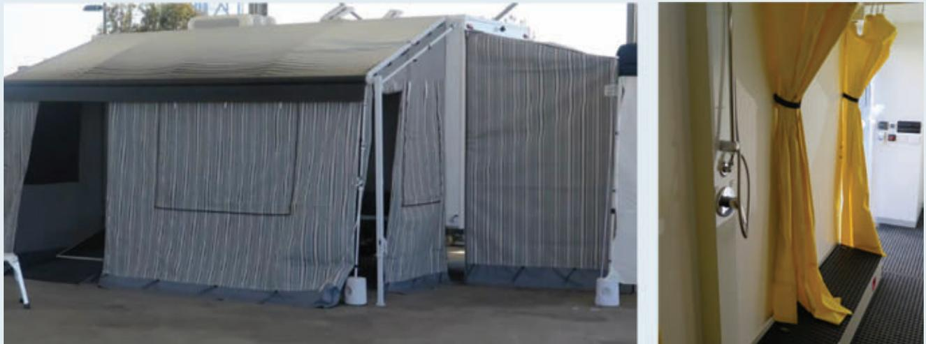
(2) QFES purpose-built decontamination trailers with (left) external awnings and (right) internal showers.
